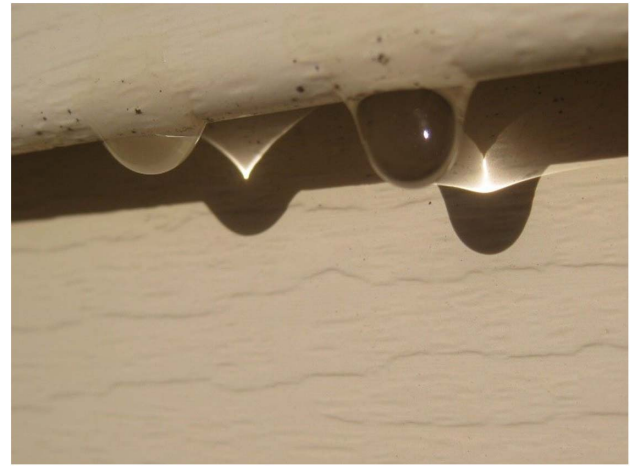
Fig. 8. Small hanging water drop and a very large hanging drop, and their near-zone transmission caustics. The values of A and of B at the attachment of the drops to the house siding are nearly equal for both drop sizes.
