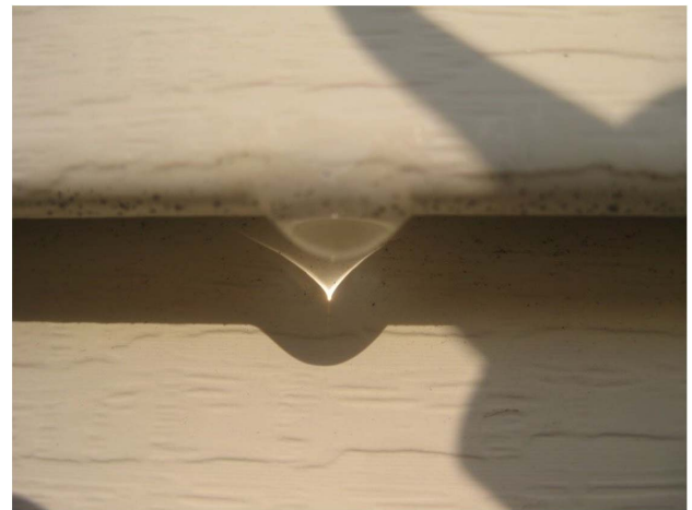
Fig. 4. Near-zone transmission caustic of a small hanging water drop. The opening angle of the caustic near its lowest point is \Psi = 59^\circ \pm 1^\circ .
