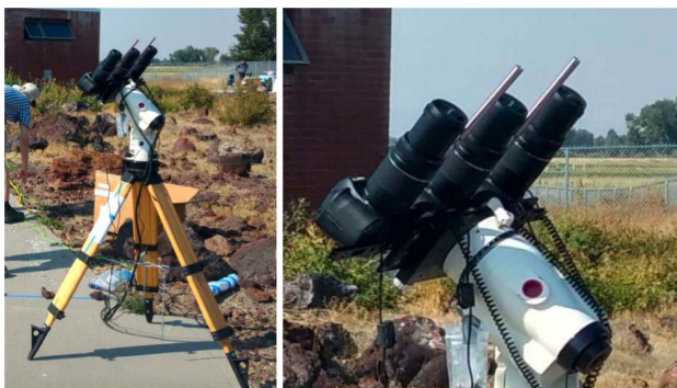
Fig. 1. Photo of the LEIPo instrument with protective lens caps instead of the polarization filters.
