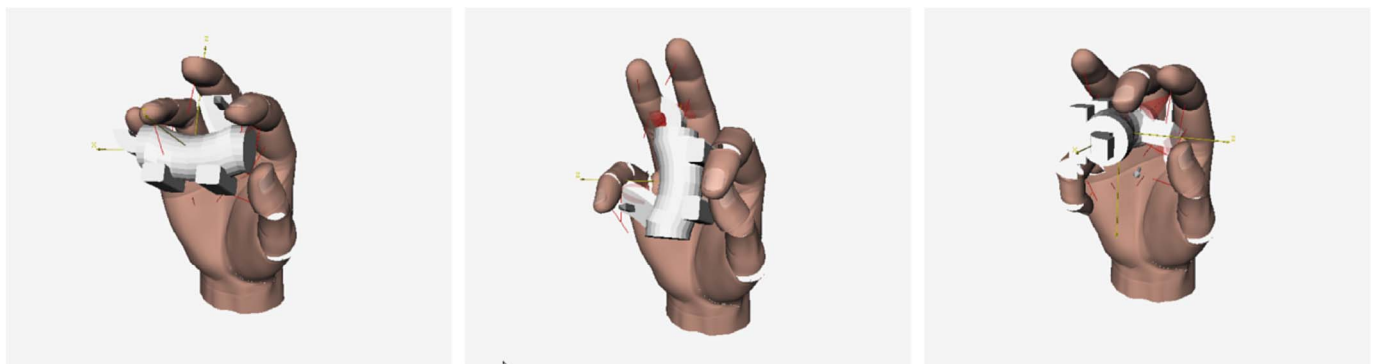
Figure 2. GraspIt! simulates a human hand. Here the hand is grasping an object at three different orientations. Reprinted from Erdogan, Yildirim, and Jacobs (2015).
