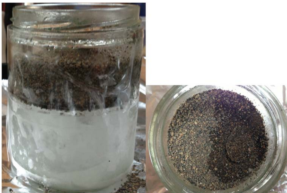
Fig. 13. Hot 250 °C basaltic tephra on top of -10 °C ice in a jar. a) Side view, glass is protected by clear tape to prevent breakage. b) Top view showing wetting the surface by escaping steaming fluids. No water layer formation was observed until the tephra cooled completely.
