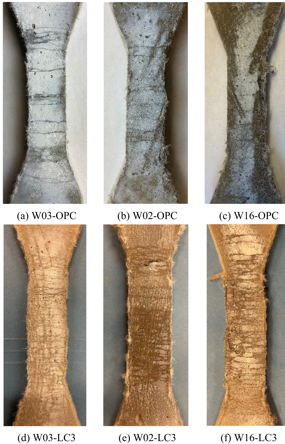
Fig. 7. Crack patterns of uniaxial tension specimens.
