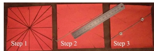
Figure 3: Stitched stretch sensor fabrication sequence (chainstitch on 4-way fabric, 60° shown). Adapted from [21]
