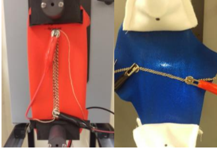
Figure 4: (Left) 4-way knit, 0° Coverstitched Sensor, 0° Force (Right) 2-way knit, 60° Chainstitched Sensor, 60° Force
