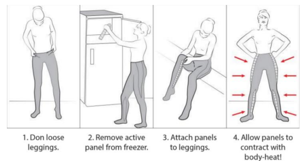
FIGURE 2: LOW-TEMPERATURE-ACTUATED SMA COMPRESSION GARMENT THAT ACTIVATES AT ROOM/BODY (ORIGINALLY APPEARED IN GRANBERRY ET AL) [10].
