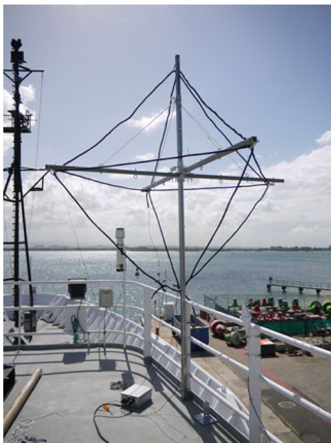
A VLF/LF antenna stands mounted on the National Oceanic and Atmospheric Administration's R/V Ronald H. Brown, while the ship was docked in Puerto Rico. Credit: Morris Cohen
