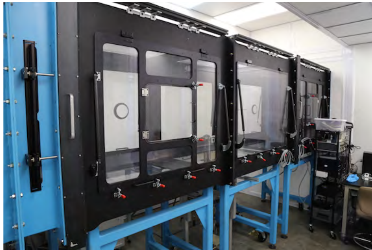
Fig. 7 Photograph of test section, looking from the downstream end. The entire test section is enclosed in “the White House” which can be used as a Biosafety-II room during animal flight testing. One of the adjustable pressure-equalization slots is visible at the far left side of the photo.
