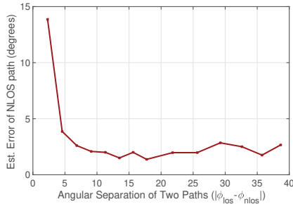
Figure 16: The estimation error of the reflected path as a function of inter-path angular separation.
