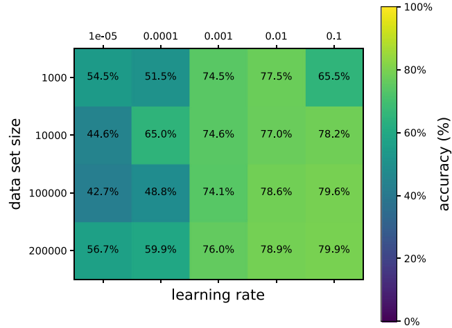
Fig. 40. Grid search results for the test set accuracy of the DNN for the SUSY problem as a function of the learning rate and the size of the dataset. The data used includes all high- and low-level features.
