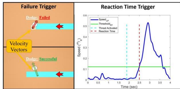
Fig. 3. Examples of the failure and reaction time triggers. The left panes represent a top down view of what a failed (A) and successful (B) maneuver looks like. The right pane details filtered velocity data from the subject's approximated center of mass location for the reaction time calculation.
