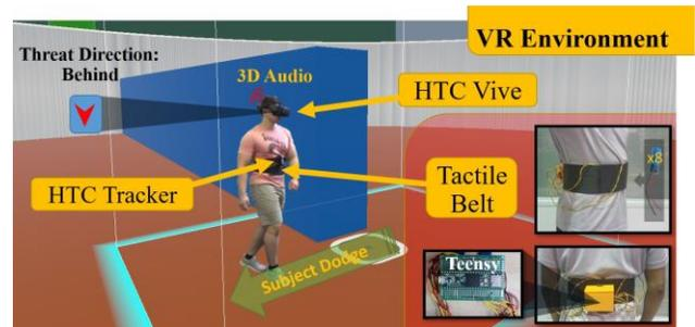
Fig. 1. Subject in custom Virtual Reality (VR) game receives audio, tactile, and visual cue of an oncoming threat from behind and physically moves to evade it. On the right is the adjustable tactile belt used.
