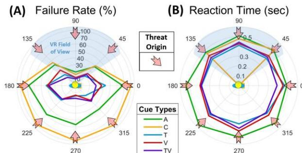
Fig. 5. Directional comparison of selected cue modes. Note that only one object was ever activated at one time. 90 degrees is the direction the subject is initially facing. This polar plot highlights the differences between failure rate (A) and reaction time (B) and their relationship to the threat's approaching direction. In both, only four conditions are displayed, missing conditions do not show any statistical difference (from T, V, TV) and are omitted.
