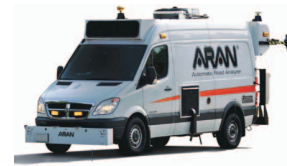
Figure 2: Automatic Road Analyzer.
