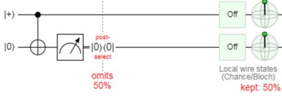
Figure 6. Verifying the classical assertion circuit using QUIRK. Although the input qubit is |+\rangle , it is projected to |0\rangle as a result of the measurement of the ancilla qubit.
