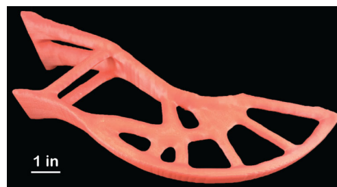
Fig. 21 Printed model of the serpentine design using the FDM 3D printing
