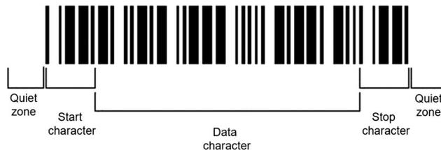
Fig. 2 Schematic view of a 1D code.
