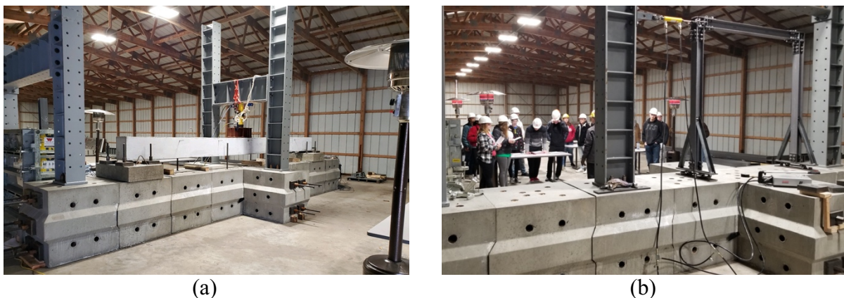
Fig. 4—The Modular Strong-block Testing System setup for (a) a beam test and (b) a frame test.
