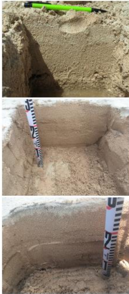
Figure 8: Representative trenches of washover fans from March 2018 (top image) and June 2019 (bottom two images). Laminations are due to compositional differences, mostly organics. Sorting and roundness are consistent throughout the trenches.
