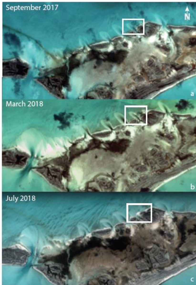
Figure 7: Channel lobe migration due to reworking by longshore currents. The top image is from September 2017, the middle image from March 2018, and the bottom image from July 2018. White boxes indicate the deposit that was eliminated by current reworking (images from Planet Team [2017]. Planet Application Program Interface: In Space for Life on Earth. San Francisco, CA. https://api.planet.com .)
