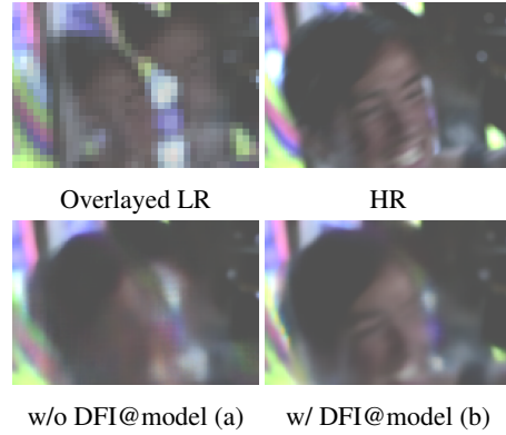
Figure 6: Ablation study on feature interpolation. The naive feature interpolation model without deformable sampling will obtain overly smooth results for videos with fast motions. With the proposed deformable feature interpolation (DFI), our model can well exploit local contexts in adjacent frames, thus is more effective in handling large motions.
