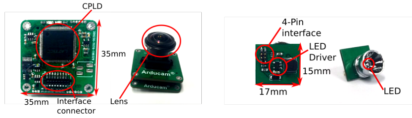
Figure 2: The major components of the IceCube Upgrade camera system. Left: A photo of the camera module, consisting of a CPLD board with SPI interface connector and an image sensor board with a lens and its mount. Right: A photo of the illumination module with a LED, LED driver, and interface connector.
