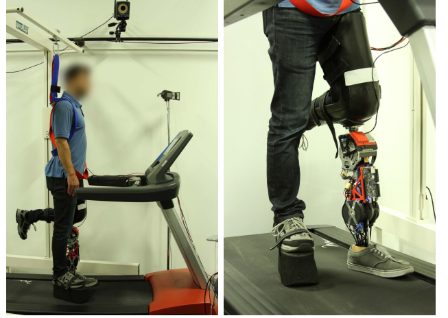
Fig. 14. Experimental setup for able-bodied walking experiments. The image on the left shows the subject, safety harness, treadmill, and sound level meter. The image on the right shows how the prosthetic leg was connected to the bypass adapter, and how it was attached to the subject's leg.
