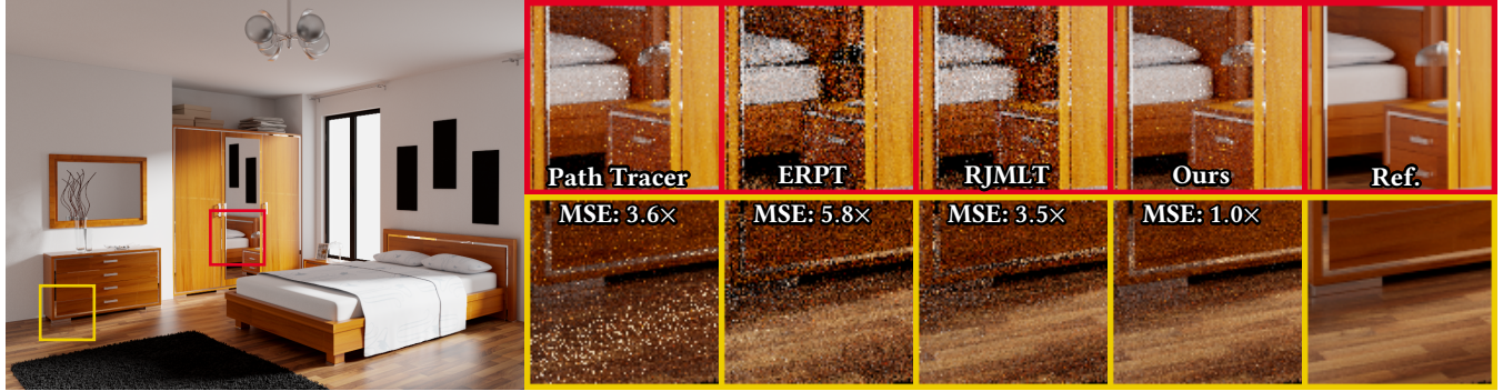
Fig. 1. For this indoor scene lit by a sun/sky environment emitter, path tracing resolves most of the lighting well, but introduces high variance in the reflective caustic cast by the mirror. ERPT and RJMLT resolve the caustic better, but do not handle diffuse lighting well and introduce noise and temporal flickering. Our method uses MLT to only resolve the difficult paths using bidirectional path tracing, and handles everything else with path tracing, leading to significantly improved MSE (relative MSE shown in insets) and vastly reduced temporal flickering (see Fig. 5). Scene ©SlykDrako.
