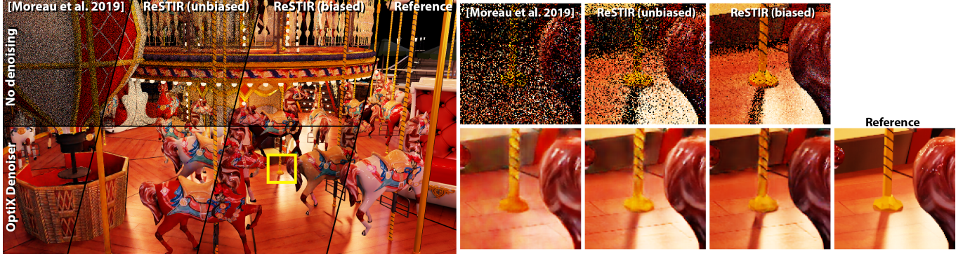
Fig. 2. While existing denoisers (e.g., Chaitanya et al. [2017]; NVIDIA Research [2017]; Schied et al. [2018]) vastly improve image quality at a given sampling rate, they cannot reconstruct features that are missing from their input samples. Our work improves the sampling quality at a given computation budget, enabling existing denoisers to produce better results. Here we show Moreau et al. [2019]’s light BVH, our unbiased (Section 4) and biased (Section 3) methods with and without the OptiX denoiser [NVIDIA Research 2017]. The AMUSEMENT PARK’s carousel image is rendered in 42 ms at 1920 \times 1080 resolution (without denoising) with 3.4 million animated lights. Carousel ©carousel_world
