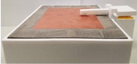
Fig. 6. Fabricated patch antenna with integrated slot on test stand to apply and remove the short across the slot.
