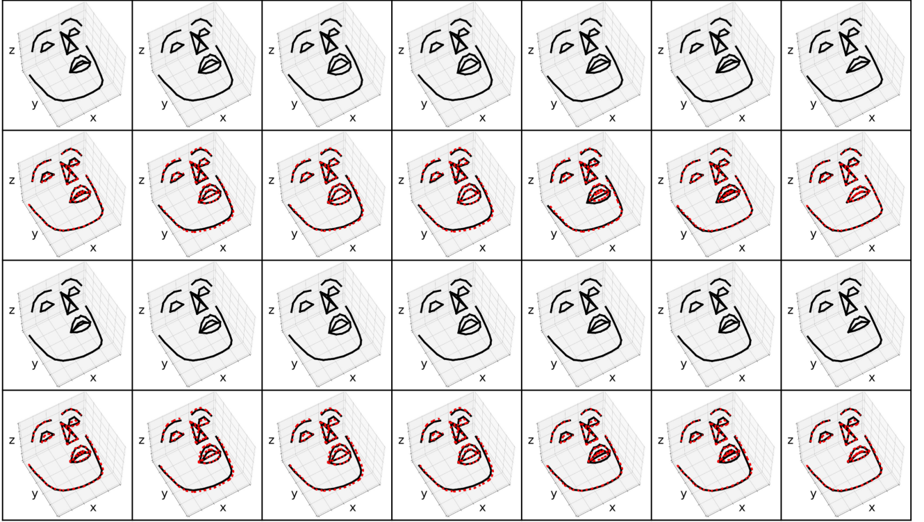
Fig. 7. The example output showing the pronunciation of the word “ash”. The speech sample was taken from STEVI corpus. The first row shows the result generated by ID_CNN . The second row shows the comparison of the result generated by ID_CNN and the ground-truth (dotted red line). The third and fourth rows show the result generated by ID_CNN_TC and comparison with the ground-truth (dotted red line). Columns show every three frames.
