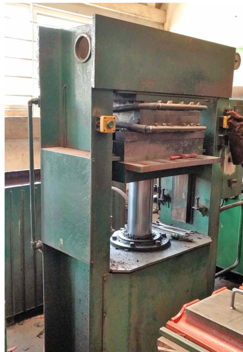
Fig. 4 Photo of tile forming press used at Resintile
