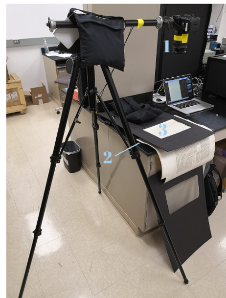
Fig. 1. Prototype of the acquisition system. The document (3) is placed on a brand light table (2) and a camera (1) captures the light passing through it. The brand light table (2) is barely visible on this picture since the document (3) is on top of it.
