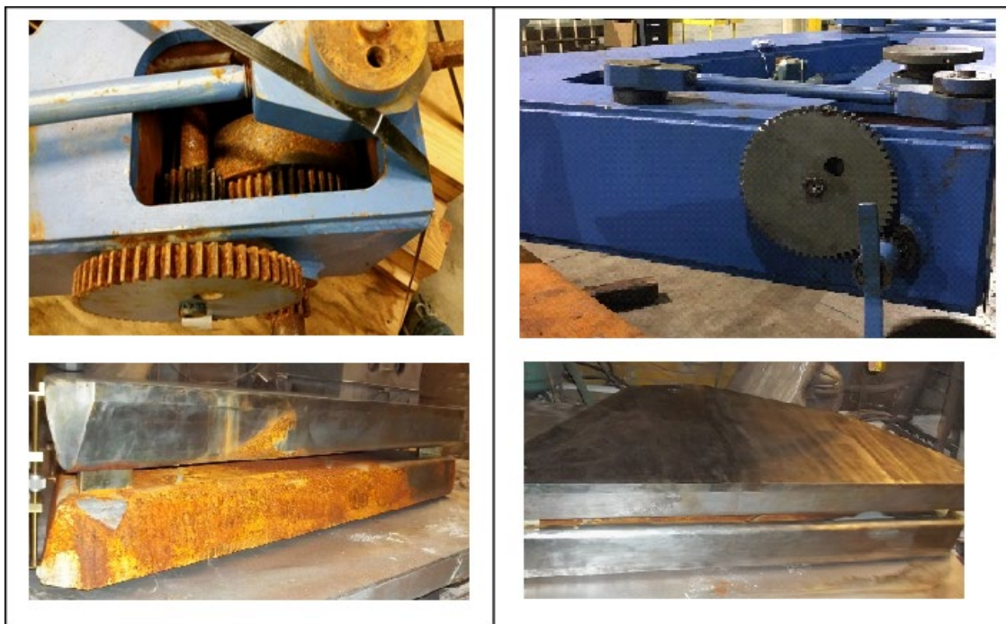
Figure 3: (Color online) (Left) Components of the spectrograph exhibiting significant rust and corrosion as they arrived at Notre Dame. (Right) The same components after refurbishment in 2017.
