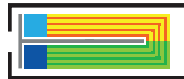
Fig. 4. A sketched illustration of the object arrangement used in proving that CRP is NP-hard to solve optimally.
