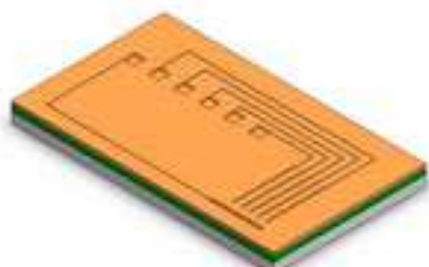
d. Ti/Au deposition
