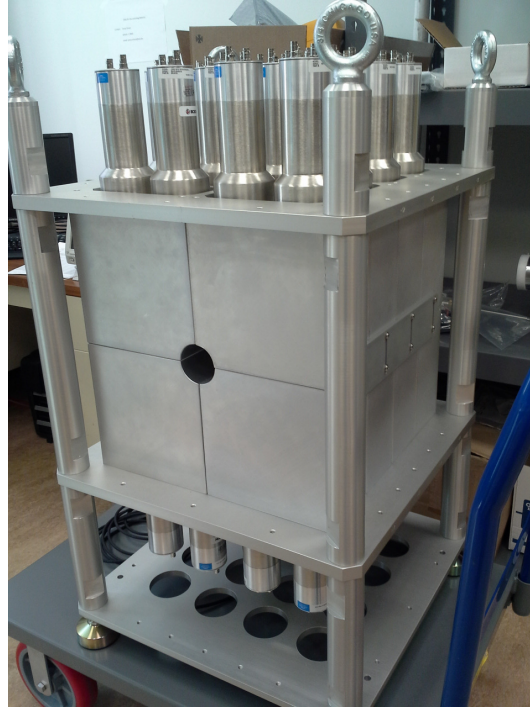
Figure 2. HECTOR: High Efficiency TOtal absorption spectrometeR.
