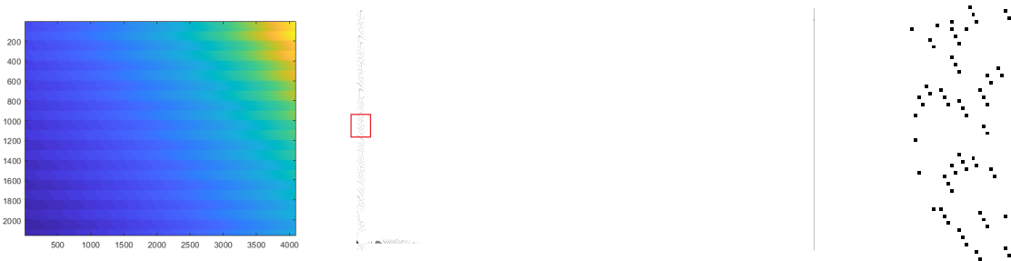
Fig. 12. Left: Ground truth image. The color assigned to each pixel corresponds to the depth of the scene along that camera ray. Center: Binary image showing the comparison between the depth map errors of each reconstruction approach. Pixels painted white are pixels for which the superresolution approach has a lower reconstruction error than the traditional temporal approach. Right: Inset showing a detail on the pixels near the edge of the image (marked by the box in the middle image) where superresolution is not as effective.
