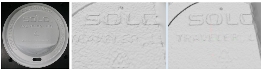
Fig. 14. Left: Scanned object. Center: Mesh reconstructed via the traditional approach. Right: Mesh reconstructed via the proposed approach.
