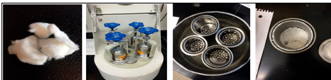
Figure 1. The cellulose pulp, ball mill, steel jars and balls, and powdered cellulose (left to right).
