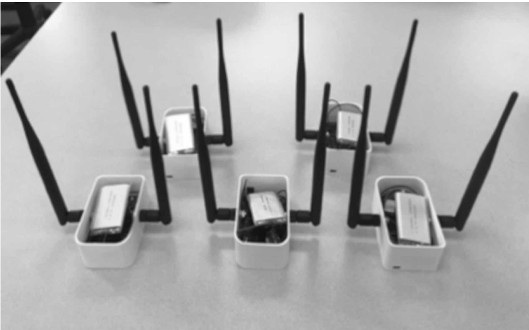
Figure 7. Developed Beaglebone platform (user0, user1, user2, user3, and user4)
