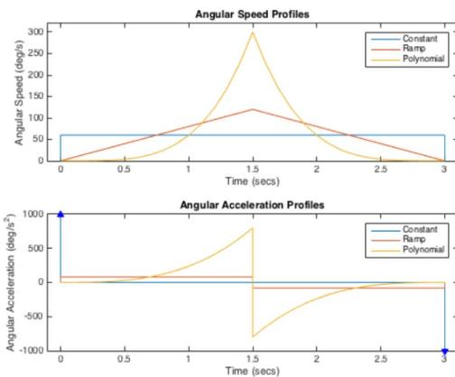
Figure 7. The speed profiles used in Experiment 2 were identical to those of Experiment 1 but converted to rates of angular displacement.
