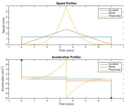
Figure 2. Three speed profiles used in Experiment 1: constant,  $s(t) = a$ ; ramp,  $s(t) = b \times t$ ; and polynomial,  $s(t) = c \times t^4$ . The acceleration and deceleration stages of each speed profile are symmetric.
