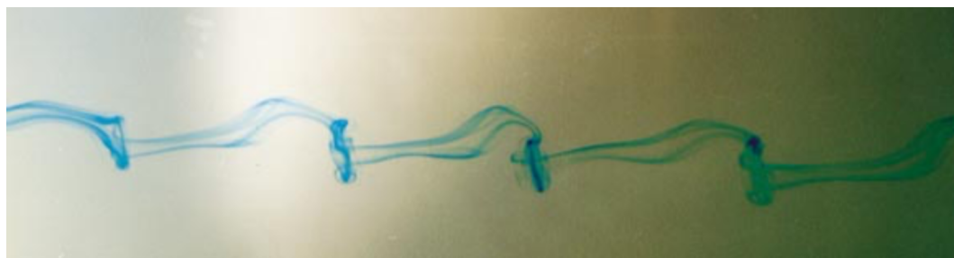
Figure 6. Experimental result 15 for the shed vortex structure of the flow past a sphere at Re = 300 .
