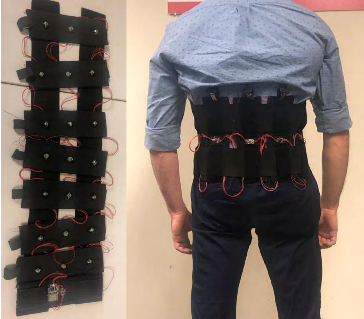
Figure 6: HaptWrap Version 2.0 consists of the following improvements: (1) Vibration motors are affixed to fabric bands, moveable along a stretchable belt to fit any waist size; (2) Vibration motors are inserted into a 3D printed structure such that the ERM's off-center mass spins orthogonal, rather than parallel, to the skin to ensure vibrations are hard to miss during ambulation; (3) Wireless communication capabilities.
