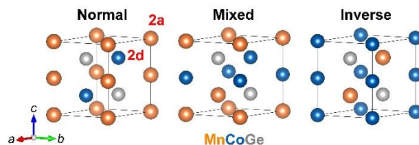
Figure 2. Models for simulating different distributions of Mn and Co atoms in the crystal structure of h -MnCoGe. Color scheme: Mn = orange, Co = blue, Ge = gray.
