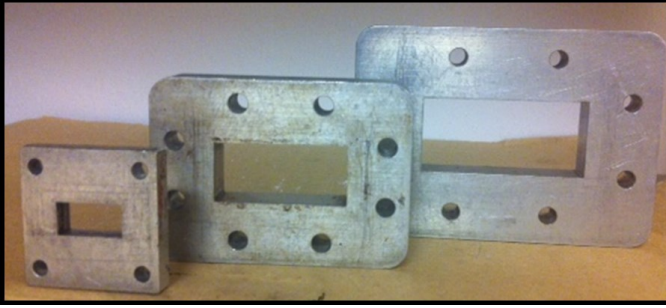
Fig. 4. Empty sample holders used for the measurement of G, C and Ku frequency bands.
