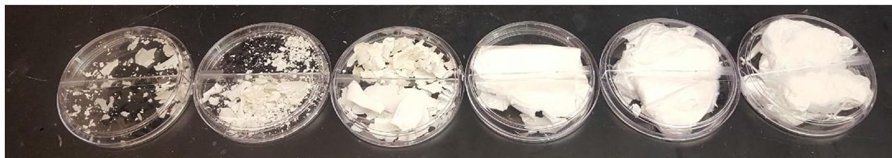
Fig. 2 Physical appearance of nanofibrous sheets consisting of PVP, CA and \text{TiO}_2 , as prepared with the same amounts of PVP and CA, with differing amounts of TIP increasing in concentration from left to right (1.0, 1.5, 2.0, 3.0, 4.0, 5.0 mL)
