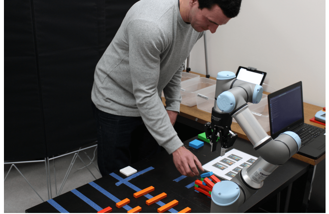
Fig. 1. In this work, participants collaborated with a UR3 collaborative robot to construct three objects under one of the three levels of task interdependence— pooled , sequential , reciprocal —while their physiological responses were recorded.
