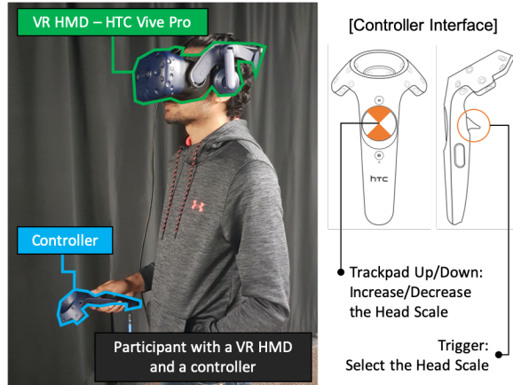
Figure 4: Annotated photo showing a participant in the experiment wearing the HMD and holding the controller during the task. The controller interface to adjust the scale of the avatar's head is shown on the right.
