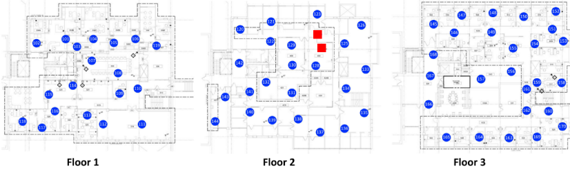
Fig. 14. The deployment of the CPSL Testbed. Blue circles denote sensors and actuators and red squares represent two access points.
