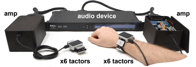
Figure 9: Syntacts In Use - This figure demonstrates a real-world implementation of the Syntacts amplifier, where it has been used to drive two Tasbi haptic bracelets [3]. A professional grade audio device (MOTU 24Ao) is connected to two Syntacts amplifier boards that have been integrated into separate Tasbi control units. Amplifier output is transmitted to each Tasbi over a multi-conductor cable. Each Tasbi bracelet incorporates six Mplus 1040W LRA tactors radially spaced around the wrist, for a total of twelve utilized audio channels. The audio device interfaces with a host PC (not shown) through a USB connection.
