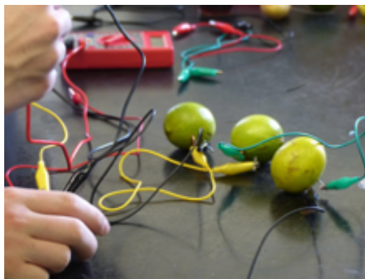
Figure 5. Fruit battery. Image courtesy of Cary Sneider
