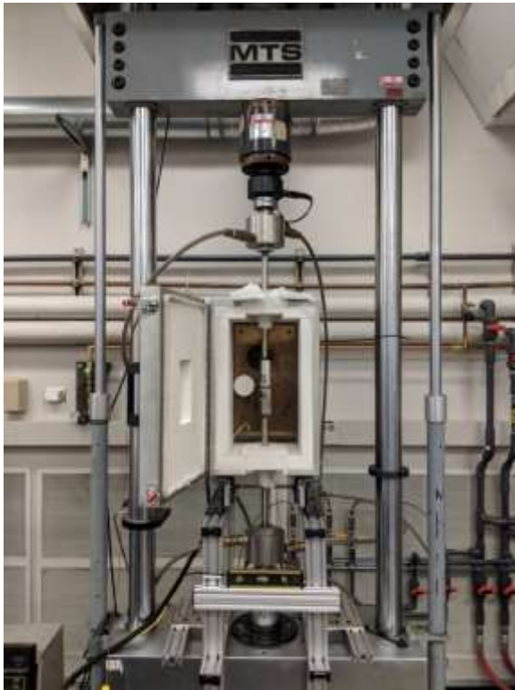
Figure 2. Specimens were pulled at elevated temperatures in uniaxial tension until rupture using the test frame shown here. Specimens were loaded in the grips and heated within the convection furnace.
