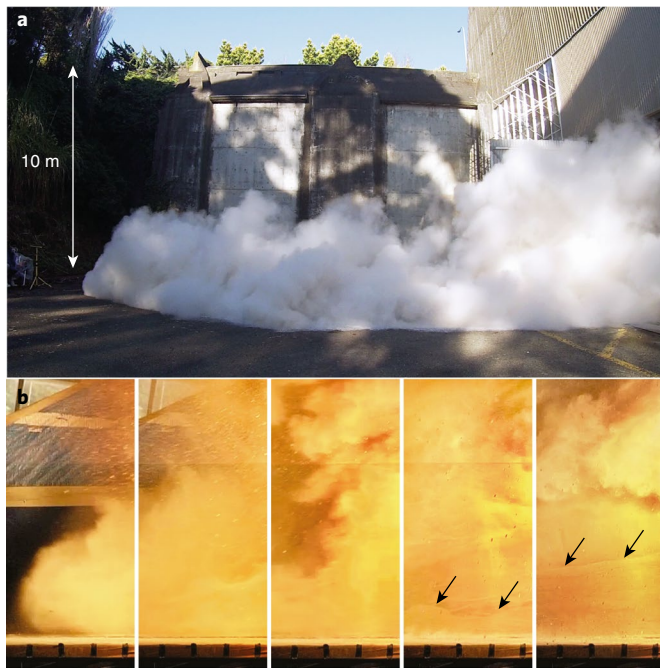
Fig. 1 | Synthesizing pyroclastic density currents in large-scale experiments. a , Oblique view of an advancing experimental pyroclastic density current at the eruption simulator PELE along the concrete pad at the end of the flume. b , Series of images of the lower 0.95 m of the flow passing an observation point at 3.2 m. Arrows highlight the boundary between the concentrated basal underflow and the dilute, turbulent over-riding ash cloud.
