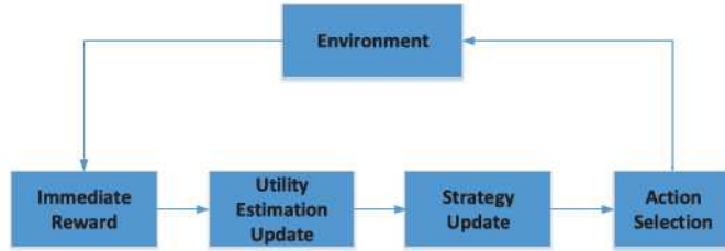
Fig. 7. The process of joint utility and strategy estimation based learning.
