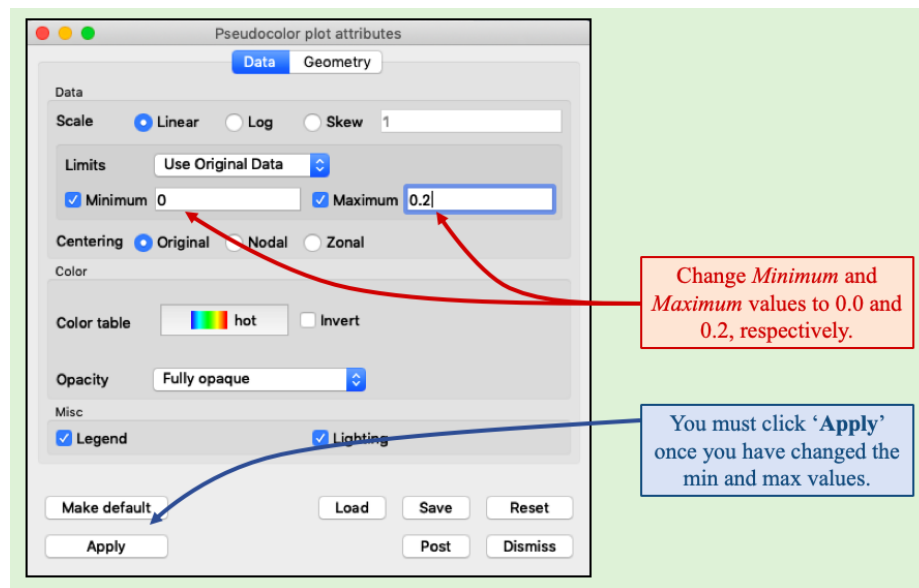
Figure 14. Changing the magnitude of velocity's colormap scaling.
