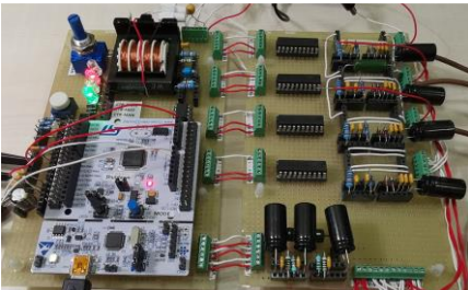
Fig. 8 Picture of the implemented power electronic interface.
